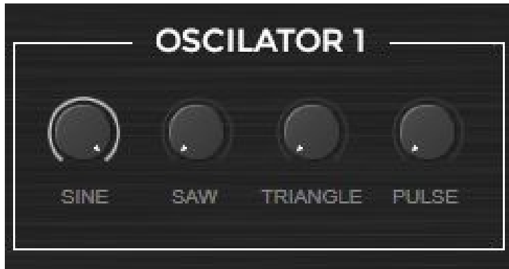
Panel detail · Oscillator 1: blending waveforms
