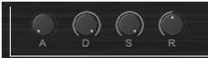
Panel detail · Local amplitude envelopes
